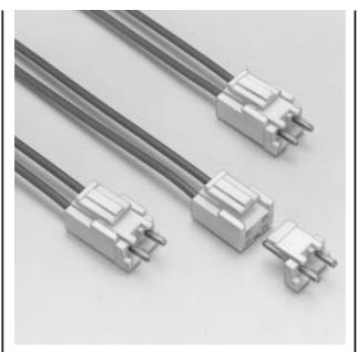
This 5.0mm (.197") pitch crimp style connector has been developed based on the box-shaped leaf contacts used successfully in the VH connector. The connector is suitable for a wide range of applications, from low-voltage, low-current signal circuits to power supply circuits requiring large currents.
