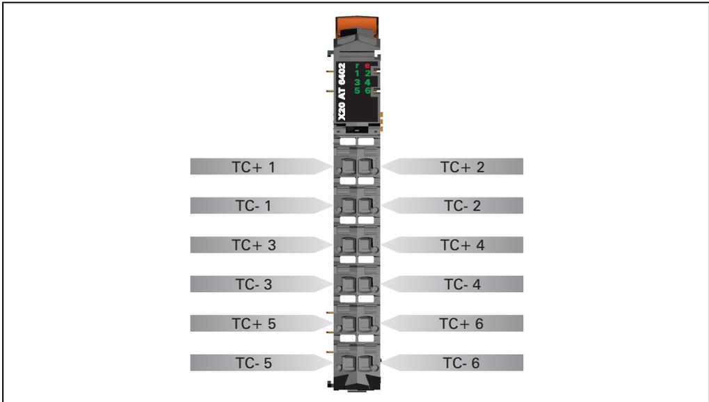
Figure 411: AT6402 - Pin assignments
