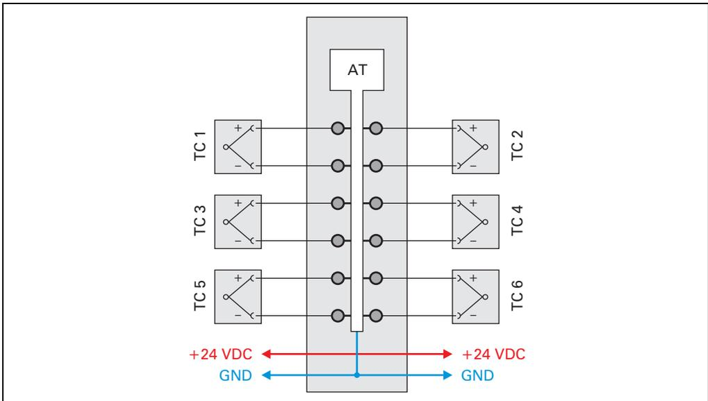
Figure 412: AT6402 - Connection example
