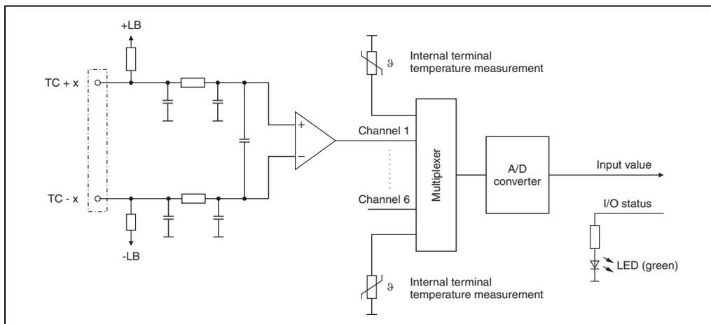
Figure 413: AT6402 - Input circuit diagram
