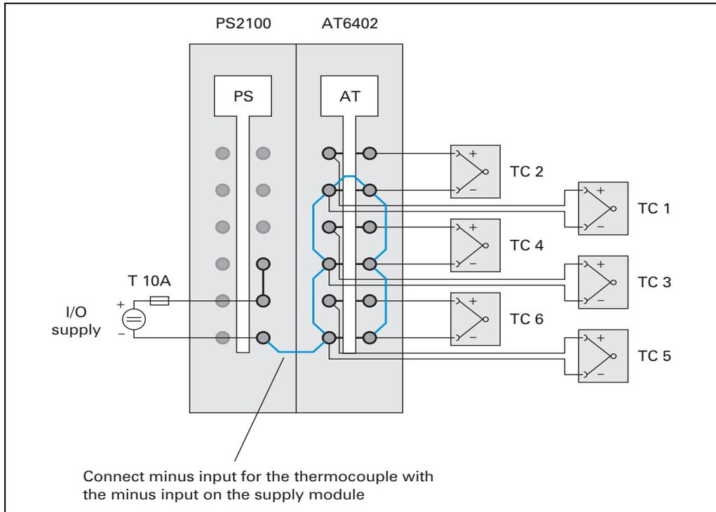
Figure 414: AT6402 - Connection of ceramic heating elements with integrated thermo elements
