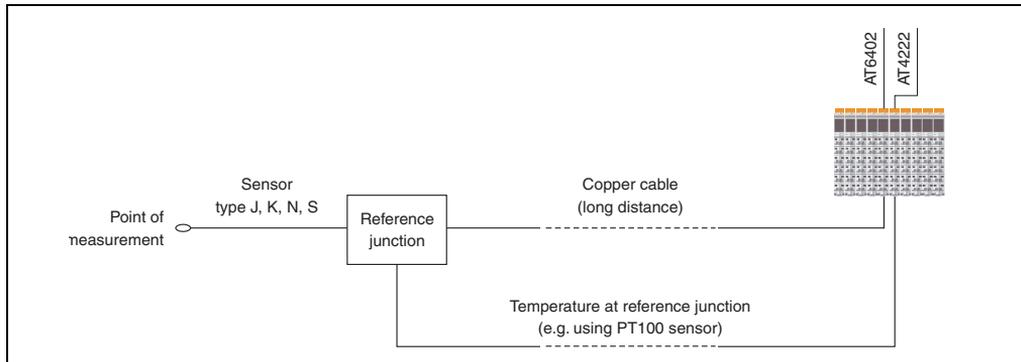
Figure 415: AT6402 - External reference junction for bridging large distances
