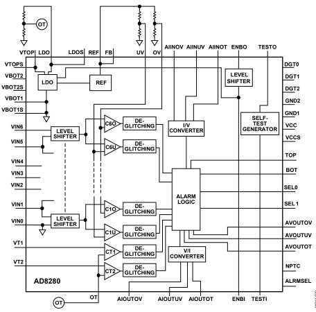
Figure 44. Functional Block Diagram
