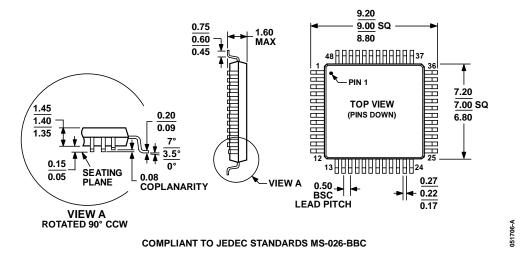
Figure 53. 48-Lead Low Profile Quad Flat Package [LQFP] (ST-48) Dimensions shown in millimeters
