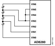
Figure 48. Four-Cell Connections for the AD8280
