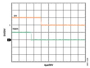
Figure 38. TESTI Edge and AVOUTxx, Self-Test Fails (Enlarged)
