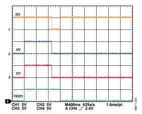
Figure 39. Alarm Condition Entering Self-Test, Part Passes Self-Test
