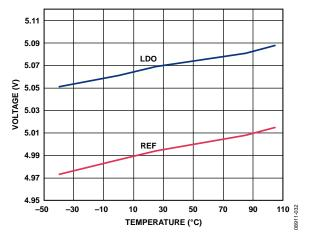
Figure 29. LDO and Reference Voltage vs. Temperature
