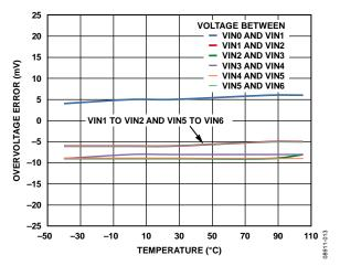
Figure 15. Overvoltage Error vs. Temperature
