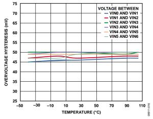
Figure 18. Overvoltage Hysteresis vs. Temperature
