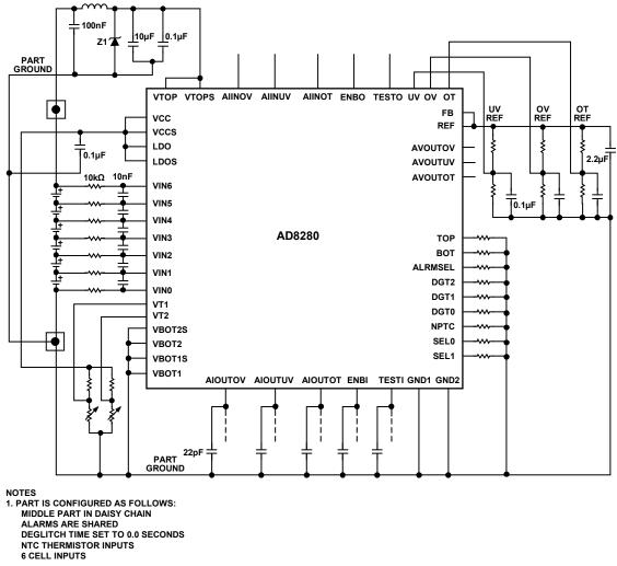
Figure 45. Typical Connections of the AD8280
