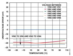
Figure 16. Undervoltage Error vs. Temperature
