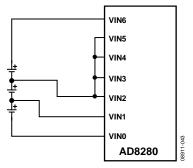
Figure 49. Three-Cell Connections for the AD8280
