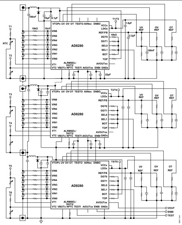
Figure 50. Typical Daisy-Chain Connections
