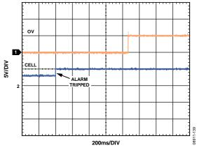
Figure 42. Cell Voltage Change to Trip Alarm, Deglitch Time = 800 ms
