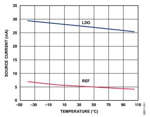
Figure 28. LDO and Reference Source Current vs. Temperature
