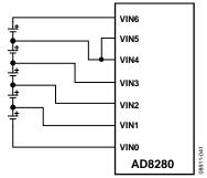
Figure 47. Five-Cell Connections for the AD8280
