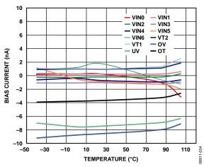
Figure 31. Input Bias Current vs. Temperature
