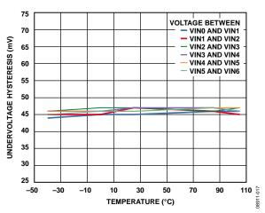
Figure 19. Undervoltage Hysteresis vs. Temperature
