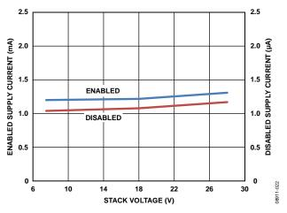
Figure 24. Supply Current vs. Stack Voltage (VIN6 – VIN0)
