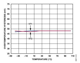
Figure 20. Overtemperature Hysteresis vs. Temperature
