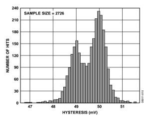
Figure 10. Overvoltage, Undervoltage, and Overtemperature Hysteresis
