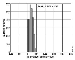
Figure 14. Supply Current, Power-Down Mode
