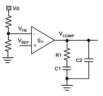
FIGURE 20. TYPE II COMPENSATOR
