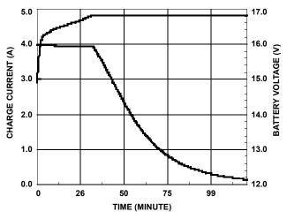
FIGURE 3. BATTERY CHARGE V-I CHARACTERISTICS
