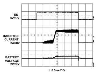
FIGURE 7. CHARGE ENABLE AND SHUTDOWN
