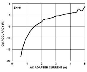
FIGURE 6. ICM ACCURACY vs AC ADAPTER CURRENT
