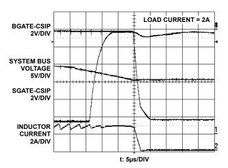
FIGURE 9. AC ADAPTER REMOVAL
