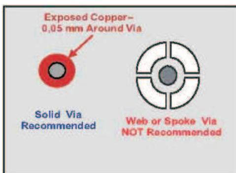
Figure 27. Thermal Via Connection at the Bottom Layer
